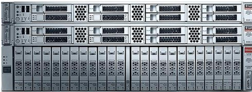
*Figure 1: ODA front panel view*
